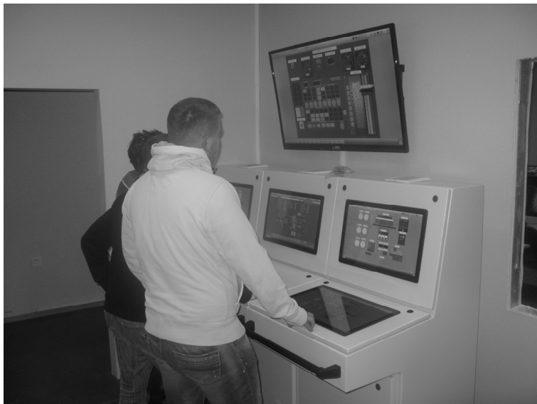
Slika 9. Transas Marine engine room simulator.
