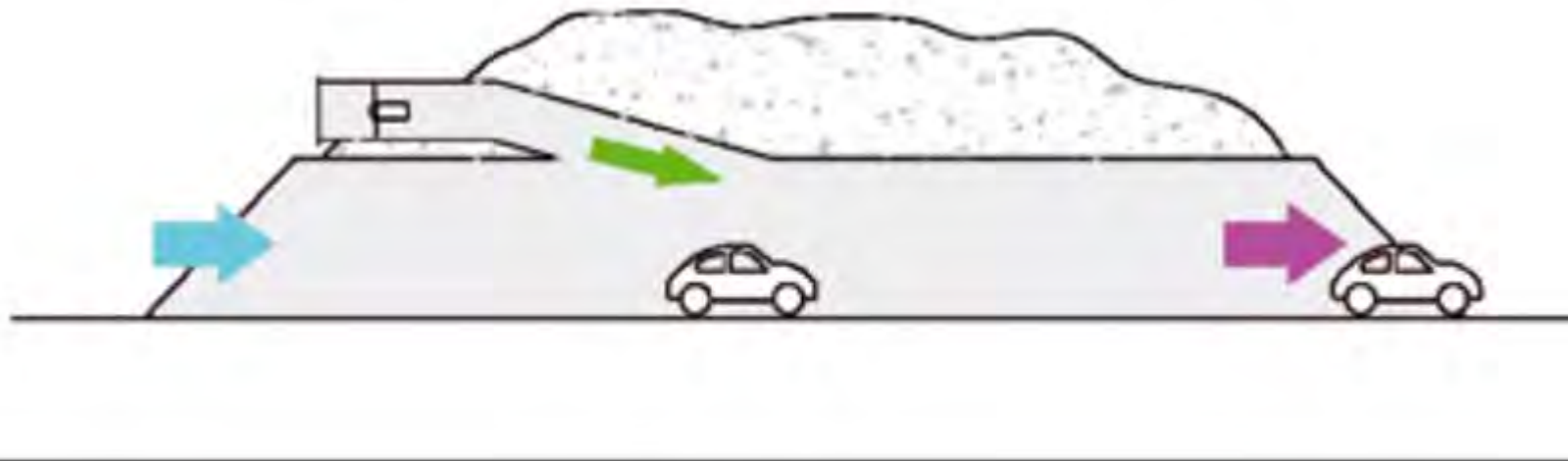
FIGURE 2 - LONGITUDINAL VENTILATION WITH SACCARDO NOZZLE
